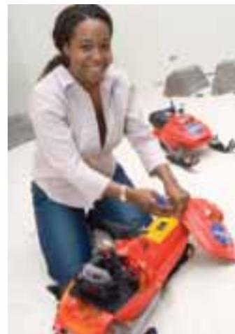
Ayanna Howard with a SnoMote, a robot designed to gather scientific data in ice environments. Photo courtesy Georgia Tech.
